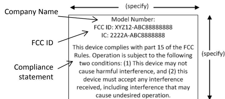
A small rectangular label diagram with the following text: 'Model Number:', 'FCC ID: XYZ12-ABC88888888', 'IC: 2222A-ABC88888888'. An arrow points from the text below to this label.
