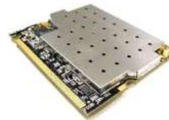
1. The radio elements must have the radio frequency circuitry shielded.
