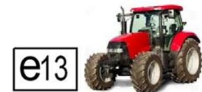
All other types of machines that do not fit the definitions for vehicles or tractors in the type approval directives will need to comply with the CE marking New Approach Directives. Common examples of these types of wheeled or tracked machines include farm equipment, construction machines, fork lift trucks, and earth moving equipment.
