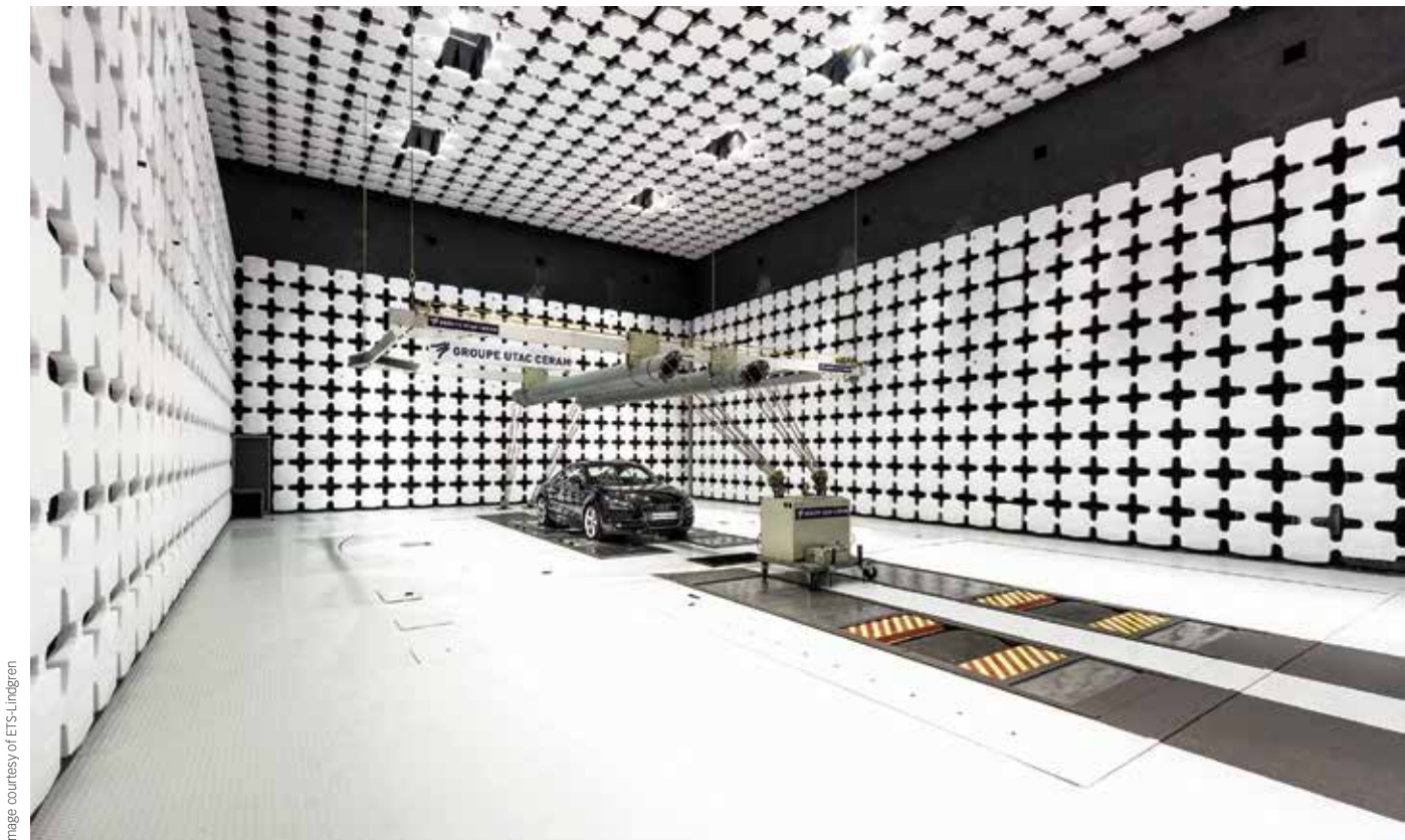
Photo 1: Automotive test chamber using polystyrene absorber
