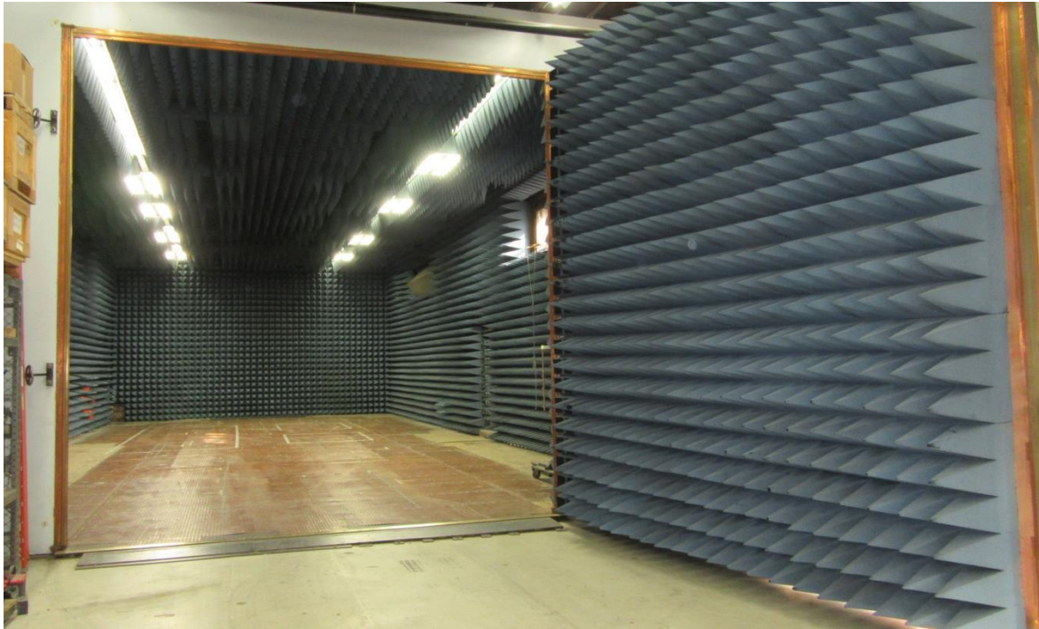
Figure – 14: Shielded Enclosure Door
