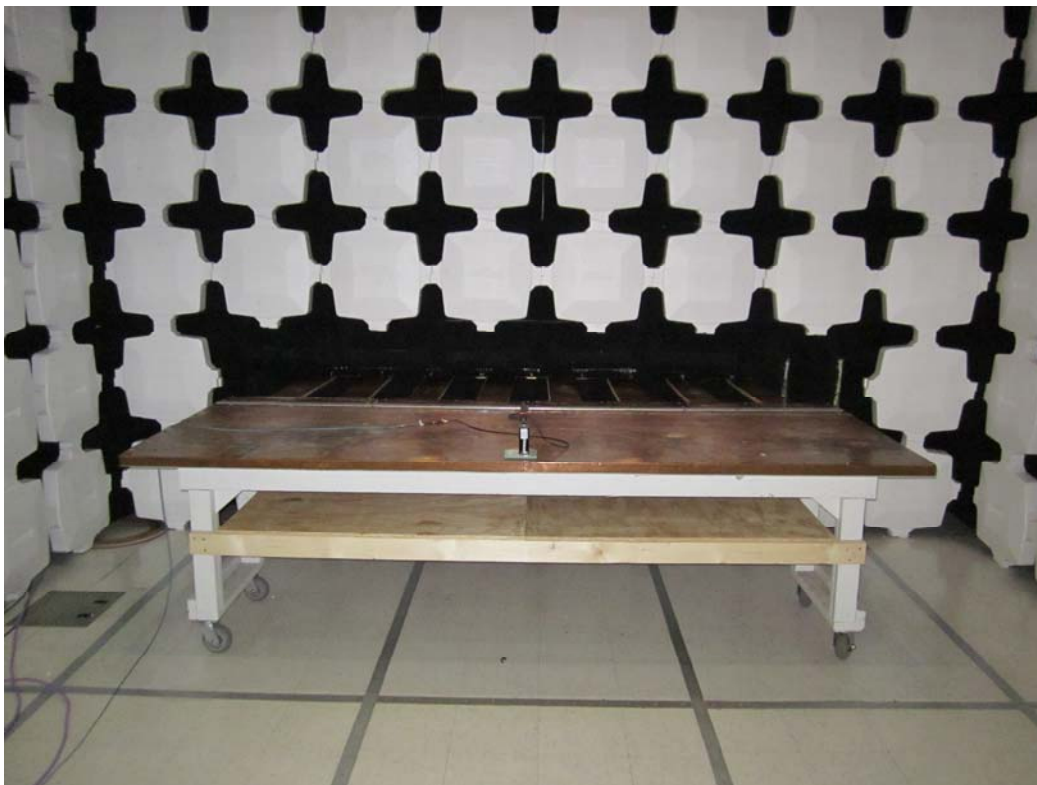
Figure – 3: Room 29F With Movable Ground Plane Shown (Test Room)
