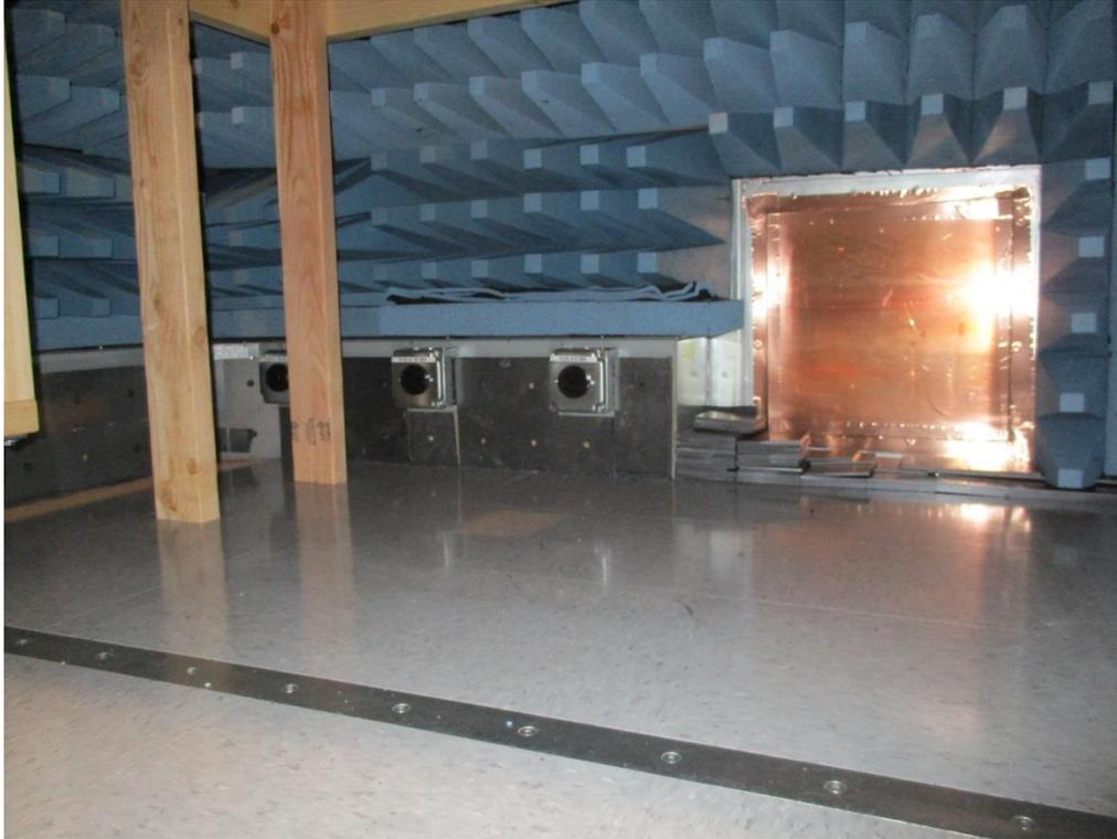
**Figure – 11: Room 12U Waveguide Opening
