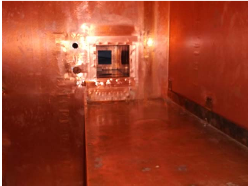
Figure – 4a: Waveguide Mounting Plate #1 w/ Universal plate and Two 2 inch copper tubes (between R23M & R23L)
