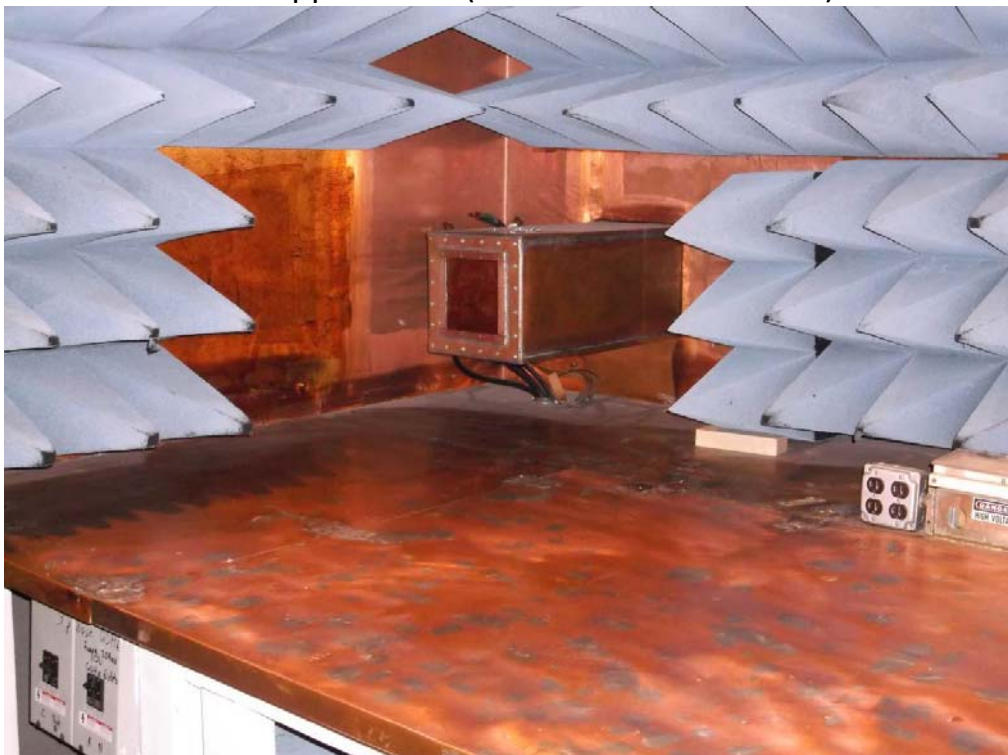
Figure – 4b: Waveguide Mounting Plate #1 w/ Universal plate and Two 2 inch copper tubes (between R23M & R23L)
